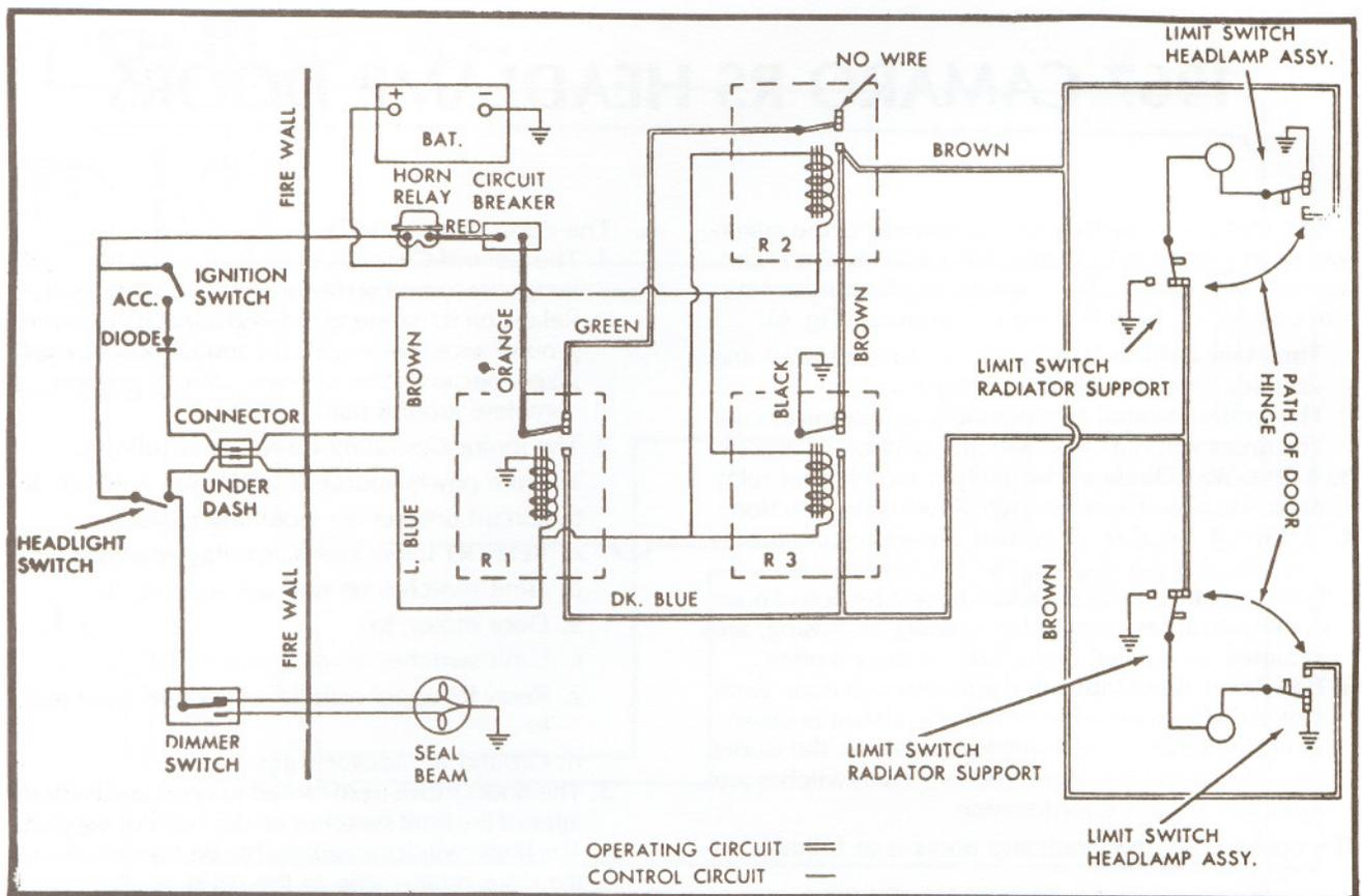
Camaro Headlamp Door Wiring—System in "Closed" Position
